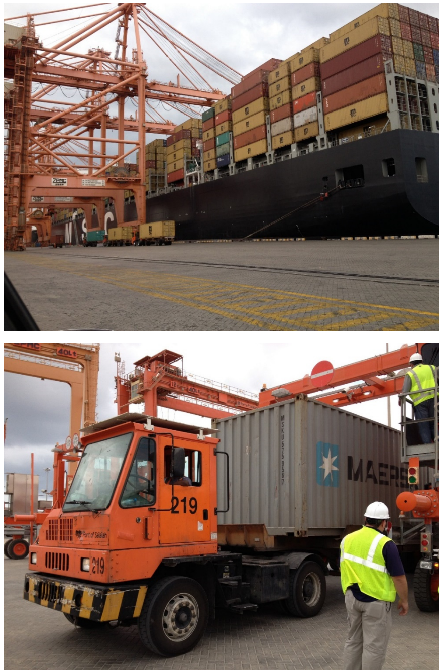
FIGURE 8-1 Mobile Radiation Detection and Identification System (MRDIS, orange structure in upper and lower images) allows vehicles with containers to pass through and be scanned for radioactive signatures (lower image). Photos are from an NNSA project at the port of Salalah in Oman where cargo is offloaded from large ships into smaller vessels appropriate for travel through the Suez Canal or taken off site via trucks. The project was a multi-lab project. Sandia was the system lead, LANL developed the sodium iodide collectors, and PNNL assisted in logistics. This is an example of deploying technologies to improve the visibility and accountability of containerized cargo to both deter trafficking of nuclear materials across borders, and improve the safety of commercial shipping. SOURCE: Photos courtesy of Dr. Rodney K. Wilson.
